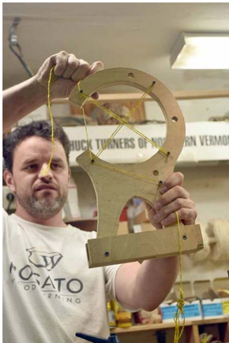
Nick demonstrates the sequence of wrapping the string around the posts.
