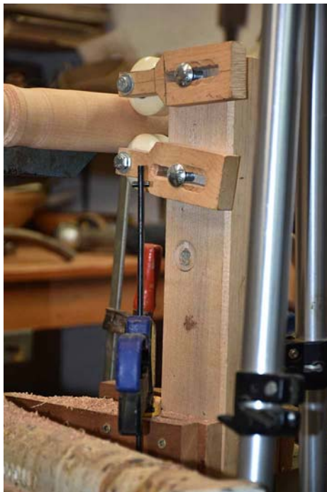
A more typical steady for use at the base of a spindle. Those are roller skate (or skateboard) wheels. Slots are cut into the mounts for flexibility. The upright must be long enough to support the contact points around the centerline of the spindle.
