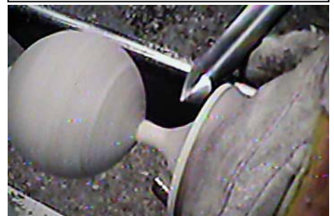
Step by step, the bead is finished off and the thin shaft is elongated by trimming down the base of the spindle.
