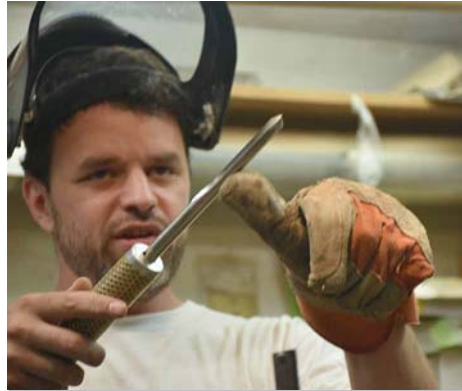
Nick uses the thumb of the supporting hand as a fulcrum to increase control over the gouge.
