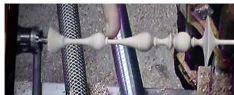
A lesser stress point where the cut transfers from the bead to the shaft more gradually.
