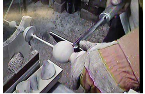
Making a cut to round off the bead. The spindle steady is supporting the already cut shaft to the left in the photo.
