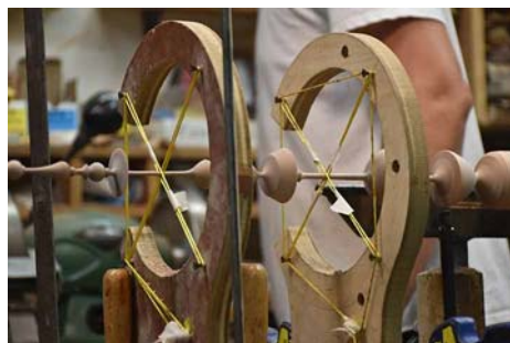
As the spindle gets more thin sections, a second or later steady is added to keep the oscillating shaft as short and stiff as possible.
