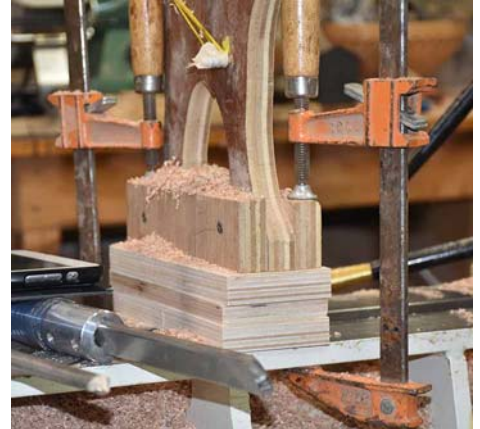
This is a detail of the mounting method of the string steady. Clamps are used to hold the base to the lathe track.
