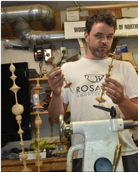
Nick explains that tremblors are long spindles with very thin sections and multiple coves and beads.
