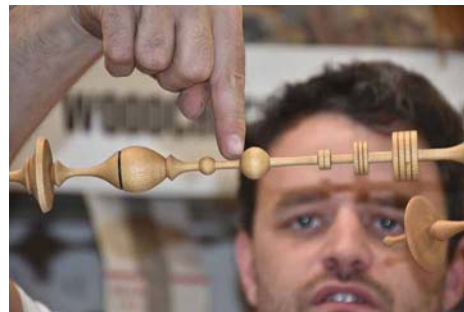
Nick points out a stress point at the base of a bead. Every place that the wood presents a sharp change in direction is a stress point, one which could cause a break.
