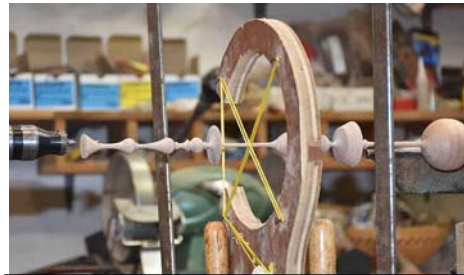
"spindle steadies" are necessary to support the work as thin sections are produced. This is an example of a home made steady using strings for maximum support of the thinnest sections.
